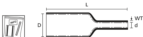
Heat Shrinkable Tubing 4:1 with adhesive
